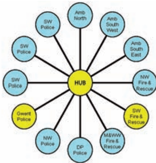
Figure 2: number of links needed to link to a central MAIT hub.
