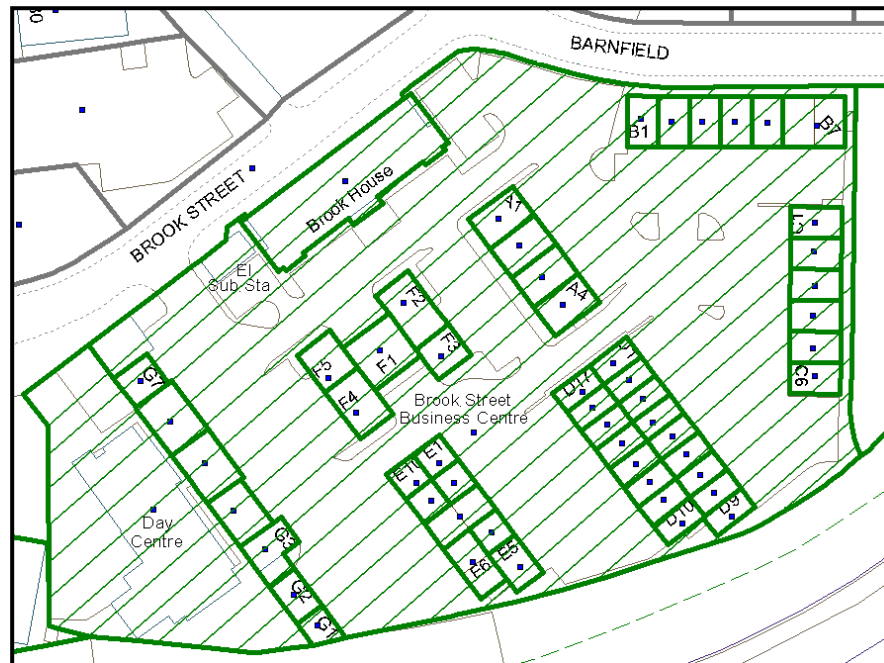
© Crown copyright All rights reserved. Sandwell M.B.C. Licence No 100032119, 2009 Figure 11 - Parent BLPU extent covers Child BLPU extents.
