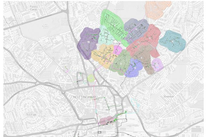
The app was created using an FME model, combining two different datasets to produce a single data source. The FME model in this instance places a layer of district heating network mapping on top of the National Street Gazetteer, creating a single source of accurate GIS data, to monitor and record where district heating systems are placed.
